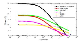
Fig 1: Solar cell efficiency as function of displacement damages
