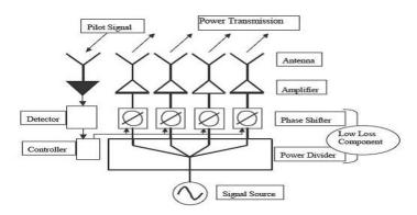
Fig 9 : Power transmission system using pilot signal.
