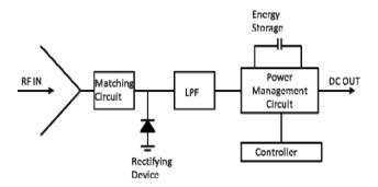
Fig 10: Schematic of antenna and associated power management circuit
