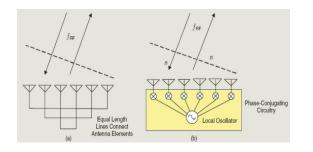
Fig 8: Retro-directive system : (a) Van atta array ,(b) phase conjugating system
